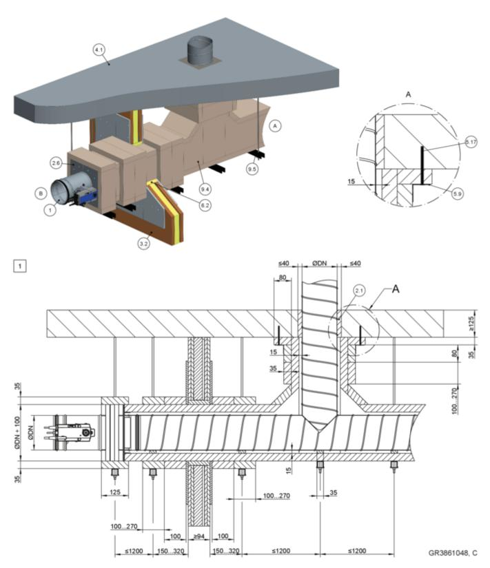
Fig. 168: Dry mortarless installation remote from solid ceiling slabs, with installation kit WE2
