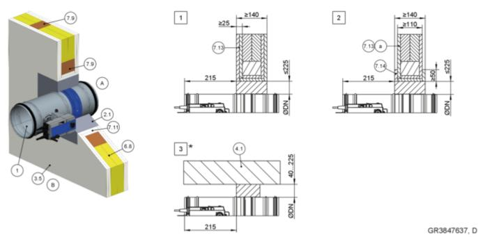
Fig. 107: Mortar-based installation into a lightweight partition wall, half-timbered construction
