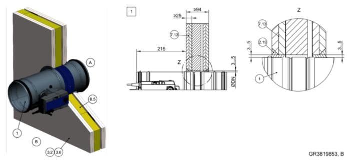
Fig. 76: Dry mortarless installation into a lightweight partition wall, without installation kit
