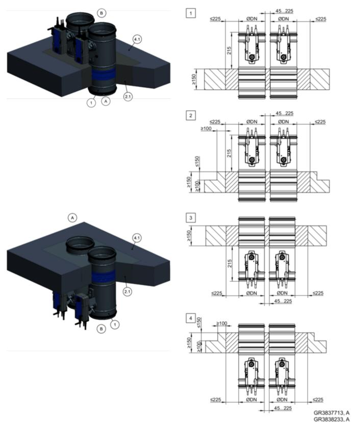
Fig. 147: Mortar-based installation into solid ceiling slab, "flange to flange", upright and suspended (also applicable for blending into the screed according to Fig. 145)
