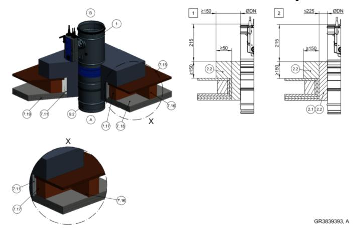
Fig. 159: Mortar-based installation in solid ceiling slab in combination with wooden beam/gluelam ceiling
