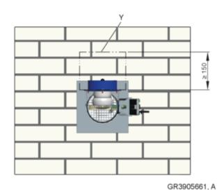
Fig. 19: FKRS-EU with spring return actuator and duct smoke detector used as an air transfer damper
