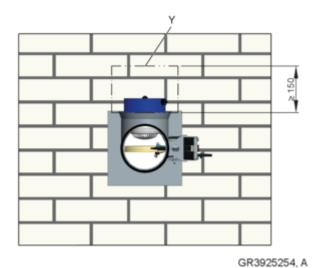
Fig. 18: FKRS-EU with spring return actuator and duct smoke detector
