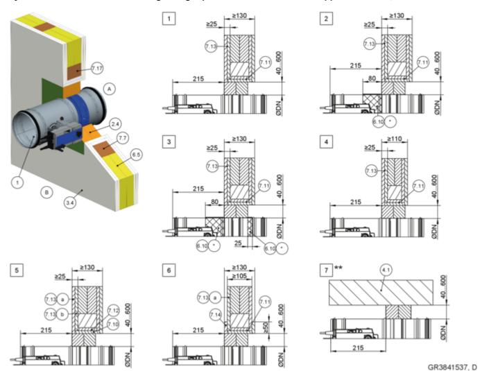
Fig. 116: Dry mortarless installation into a lightweight partition wall with timber support structure, with a fire batt
