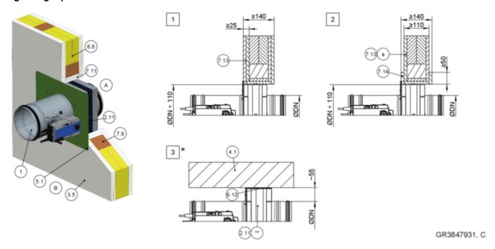
Fig. 111: Dry mortarless installation into a lightweight partition wall, half-timbered construction, using installation kit TQ2
