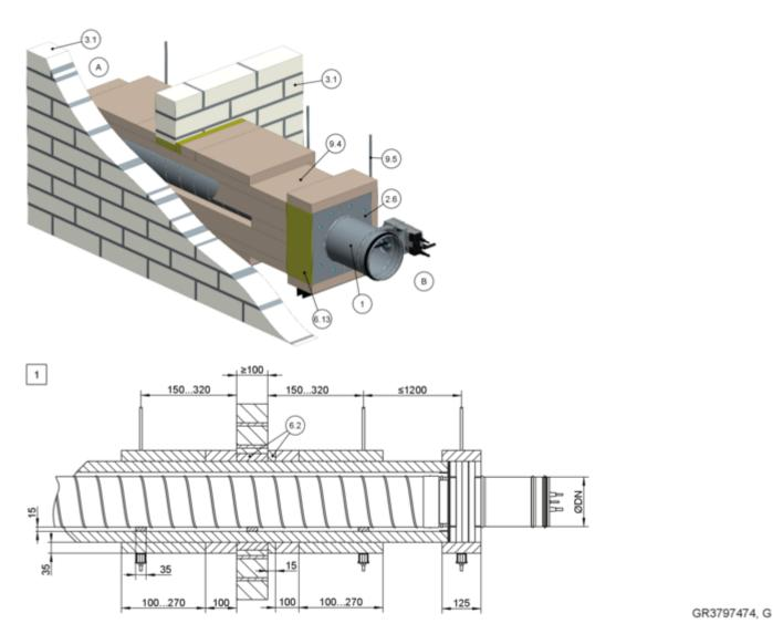
Fig. 56: Dry mortarless installation remote from solid walls with installation kit WE2 (wall penetration), three-sided cladding
