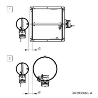
Fig. 27: Distance from the FKRS-EU to other TROX fire dampers in mortar-based installation
