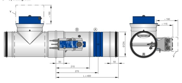
Fig. 6: FKRS-EU with Belimo spring return actuator and duct smoke detector, drawn in a round air duct (on-site)
