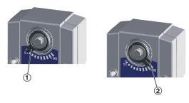
Fig. 195: Damper blade position indicator
