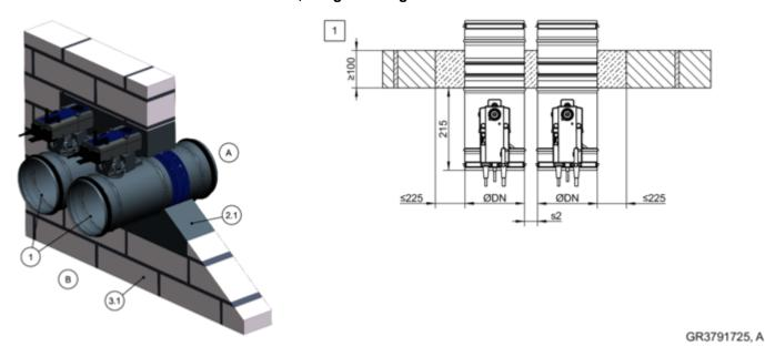
Fig. 39: Mortar-based installation into a solid wall, flange to flange, illustration shows side by side installation (applies also to installation of dampers on top of each other)
