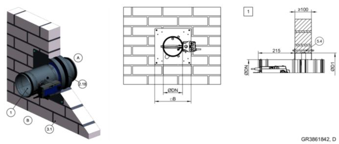
Fig. 47: Dry mortarless installation in solid wall with installation block ER
