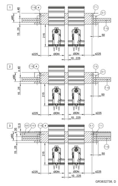
Fig. 134: Mortar-based installation into a shaft wall, flange to flange, illustration shows side by side installation (applies also to installation of dampers on top of each other)
