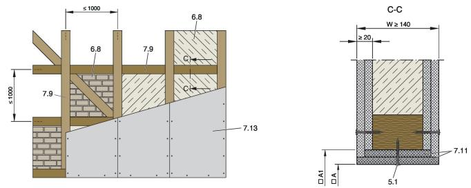
Fig. 103: Lightweight partition wall, half-timbered construction with cladding on both sides
