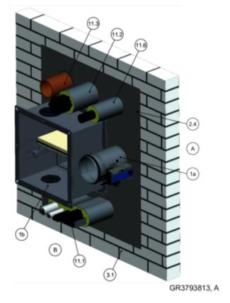
Fig. 24: Combined penetration seal (drawn solid wall)
