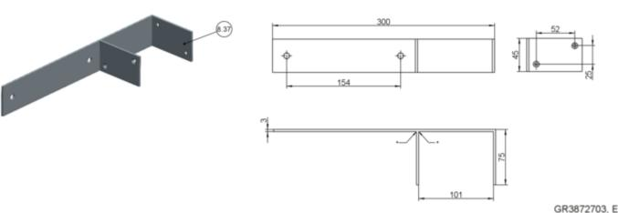
Fig. 35: Steel angle for dry mortarless installation with installation kit GL2 in lightweight partition wall if there is no rear fastening possibility
