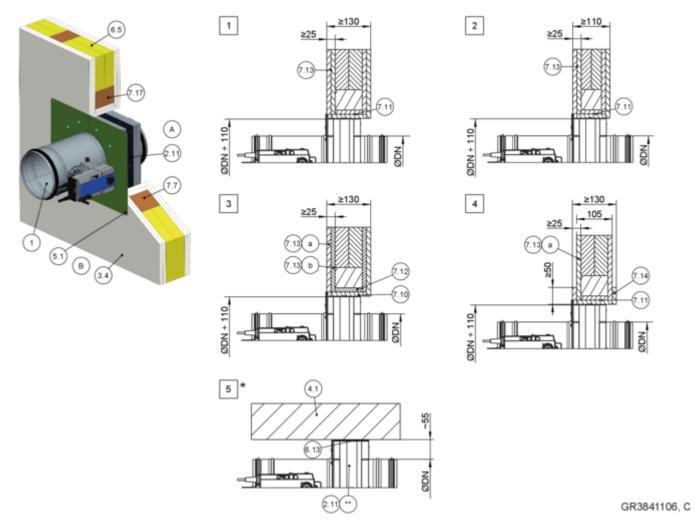
Fig. 110: Dry mortarless installation into a lightweight partition wall with timber support structure, with installation kit TQ2
