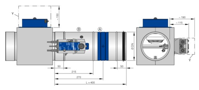
Fig. 5: FKRS-EU with Belimo spring return actuator and duct smoke detector, drawn in a square air duct (on-site)
