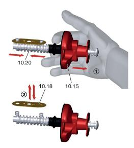
Fig. 200: Replacing the fusible link
