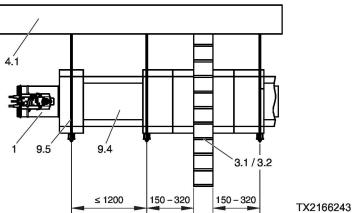
Fig. 185: FKRS-EU in a cladded duct
