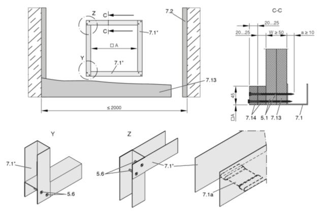
Fig. 140: Shaft wall without metal support structure and with cladding on one side
