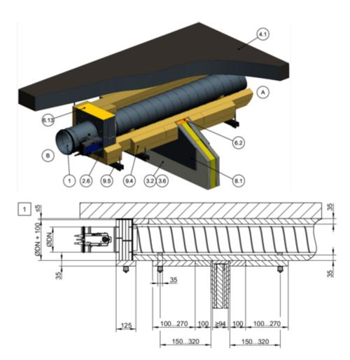
Fig. 84: Dry mortarless installation remote from lightweight partition walls with installation kit WE2 (wall penetration), three-sided cladding
