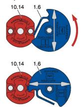
Fig. 192: Opening the damper blade
