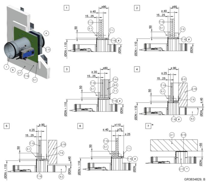
Fig. 137: Dry mortarless installation into a shaft wall with metal support structure, with installation kit TQ2
