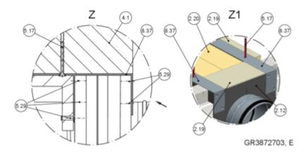
Fig. 95: Dry mortarless installation in lightweight partition wall with installation kit GL2 and steel bracket if there is no rear fixing option
