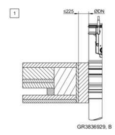
Fig. 178: Mortar-based installation into historic wooden beam ceilings, illustration shows upright installation (applies also to suspended installation)
