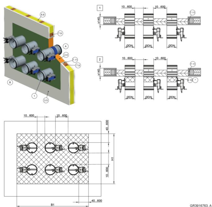
Fig. 122: Dry mortarless installation with fire batt in lightweight partition wall with half-timbered construction - multiple occupancy of an installation opening
