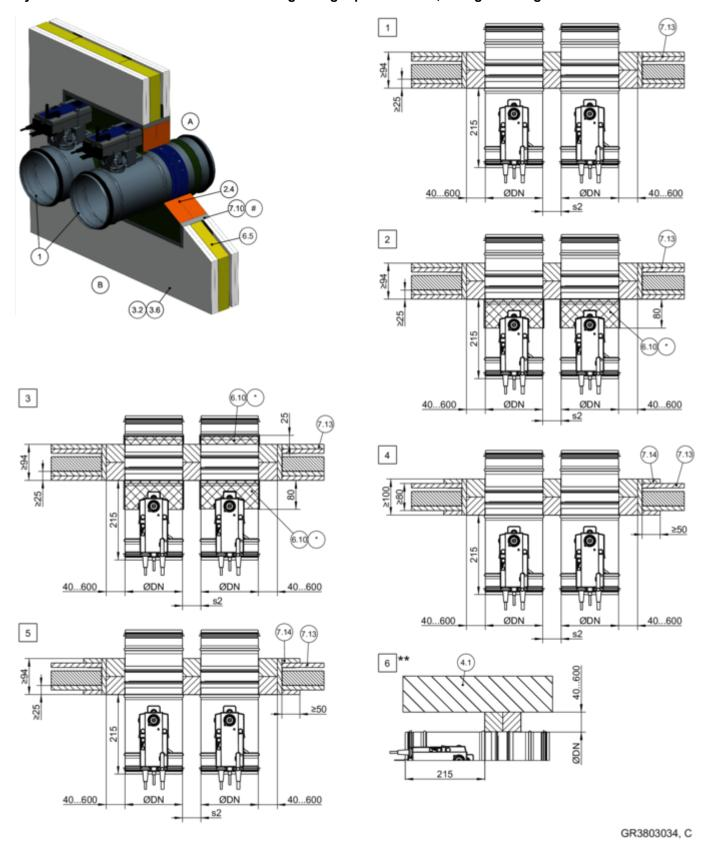
Fig. 97: Dry mortarless installation into a lightweight partition wall, with a fire batt, flange to flange, illustration shows side by side installation (applies also to installation of dampers on top of each other)
