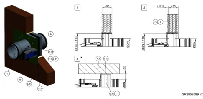
Fig. 126: Dry mortarless installation into a solid wood wall or CLT wall, with installation kit TQ2
