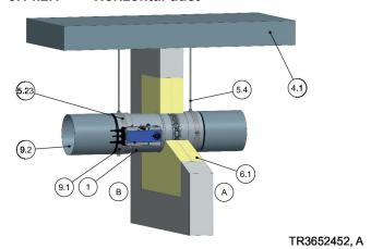
Fig. 181: Suspension system, horizontal duct
