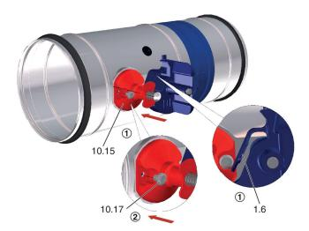
Fig. 201: Install the fusible link holder
