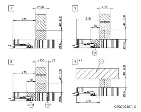
Fig. 60: Dry mortarless installation with fire batt into a solid wall
