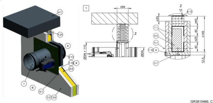
Fig. 81: Dry mortarless installation with installation kit TQ2 into a lightweight partition wall, below a flexible ceiling joint
