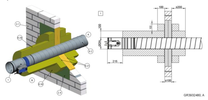
Fig. 59: Dry mortarless installation remote from solid walls with mineral wool and fire batt
