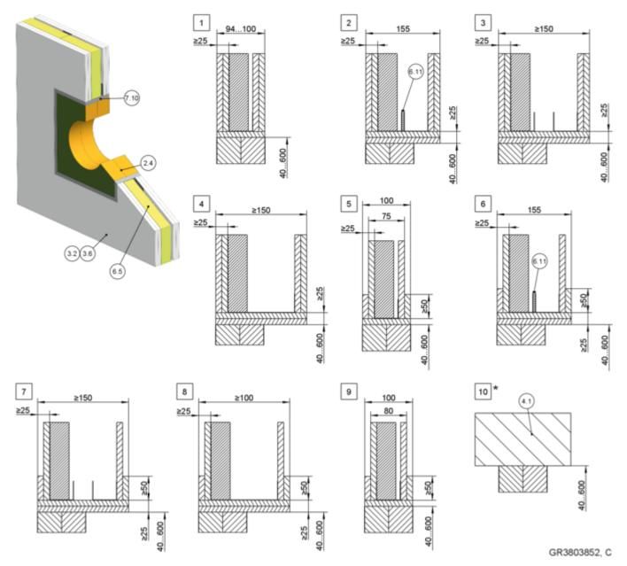
Fig. 98: Dry mortarless installation into a lightweight partition wall, with a fire batt, approved combinations for thicker walls
