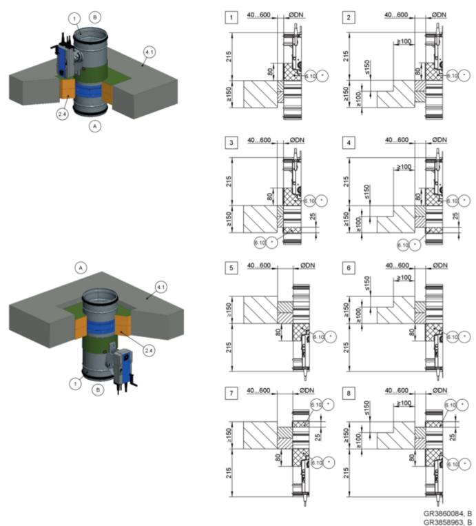
Fig. 170: Dry mortarless installation into a solid ceiling slab, with a fire batt, upright and suspended
