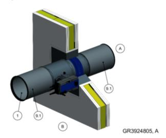
Fig. 187: FKRS-EU with flexible connectors
