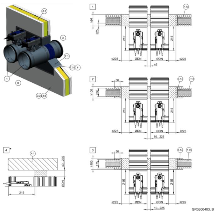
Fig. 71: Mortar-based installation into a lightweight partition wall, flange to flange, illustration shows side by side installation (applies also to installation of dampers on top of each other)
