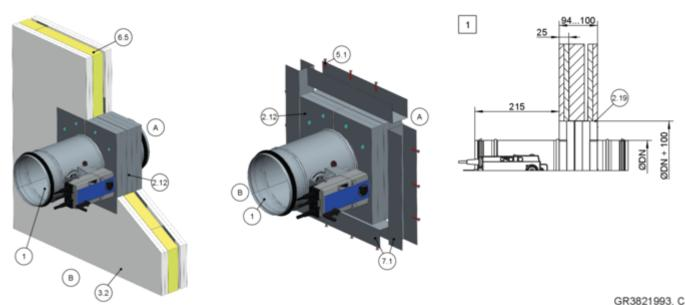
Fig. 88: Dry mortarless installation in lightweight partition wall with installation kit GL2 during wall construction
