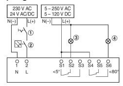
Fig. 190: Actuator connection, example
