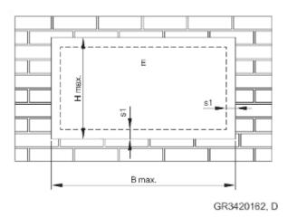
Fig. 23: Fire batt – installation in solid walls and ceilings, lightweight partition, timber stud wall, half-timbered construction and solid wood walls
