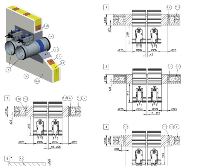
Fig. 105: Mortar-based installation into a lightweight partition wall with timber support structure, flange to flange, illustration shows side by side installation (applies also to installation of dampers on top of each other)
