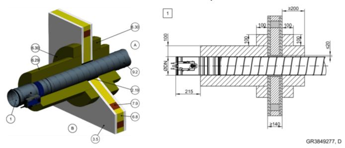
Fig. 113: Installation remote from timber frame walls with mineral wool and joint filler
