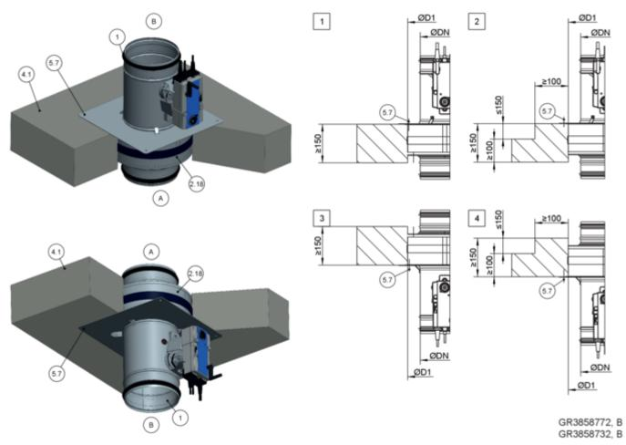
Fig. 165: Dry mortarless installation with installation block ER in solid ceiling slab, upright and suspended
