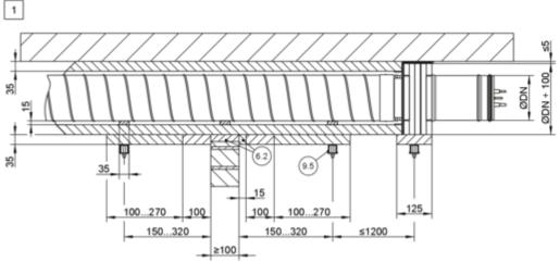
Fig. 57: Dry mortarless installation remote from solid walls with installation kit WE2 (wall penetration), two-sided cladding
