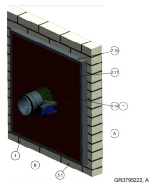
Fig. 25: Fire protection stone bulkhead (single penetration)
