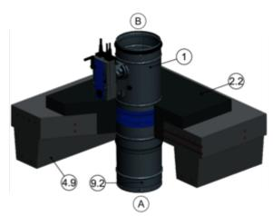
Fig. 157: Mortar-based installation in ribbed ceiling
