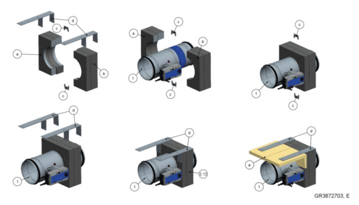
Fig. 34: Scope of supply and installation of installation kit GL2 (steel bracket and cover to be provided by customer) for dry mortarless installation if there is no ceiling fixing on the rear side
