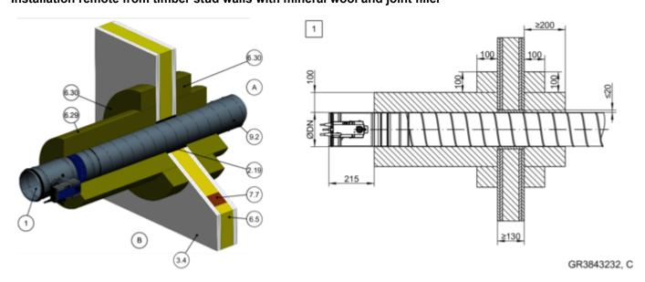
Fig. 112: Installation remote from timber stud walls with mineral wool and joint filler
