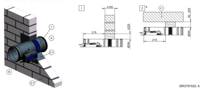
Fig. 38: Mortar-based installation into a solid wall
