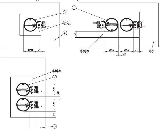
Fig. 131: Shaft walls with metal support structure – arrangement/distances
