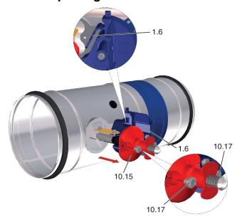
Fig. 199: Removing the fusible link holder
