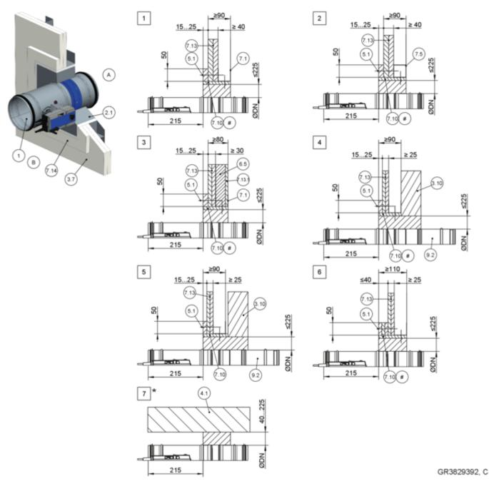
Fig. 133: Mortar-based installation into shaft wall with metal support structure
