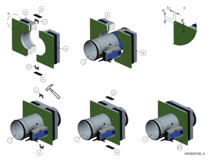
Fig. 30: Supply package and installation of installation kit TQ2 for dry mortarless installation
