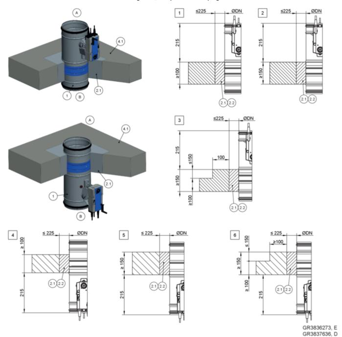
Fig. 145: Mortar-based installation into a solid ceiling slab, suspended or upright
