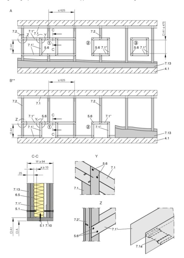
Fig. 65: Lightweight partition wall with metal support structure and cladding on both sides, explanation see Fig. 66
