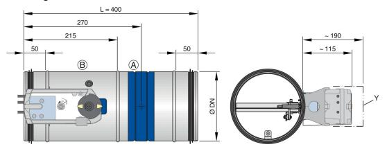
Fig. 4: FKRS-EU with Siemens spring return actuator
