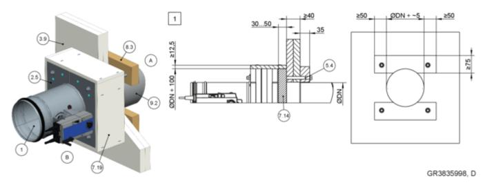
Fig. 143: Dry mortarless installation into a shaft wall without metal support structure, with installation kit WA2
