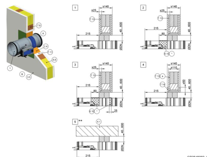
Fig. 118: Dry mortarless installation into a lightweight partition wall, with fire batt, with half-timbered construction
