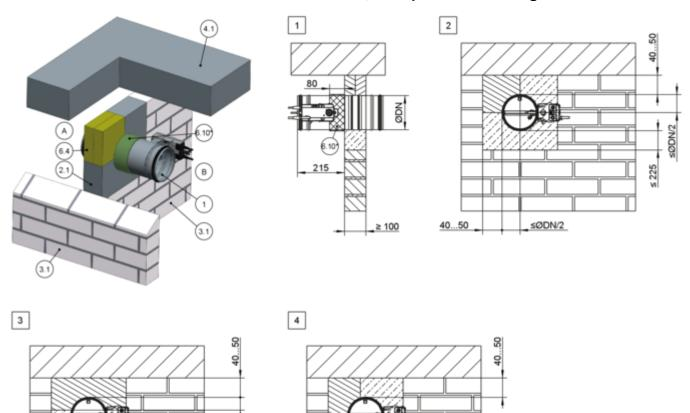
Fig. 45: Mortar-based installation into a solid wall, with partial mortaring
