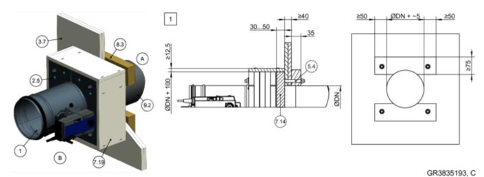
Fig. 138: Dry mortarless installation into a shaft wall with metal support structure, with installation kit WA2
