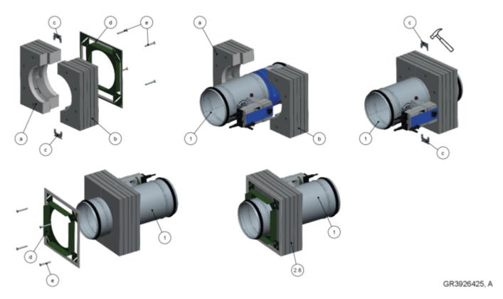
Fig. 32: Scope of supply and assembly Installation kit WE2 for dry mortarless installation
