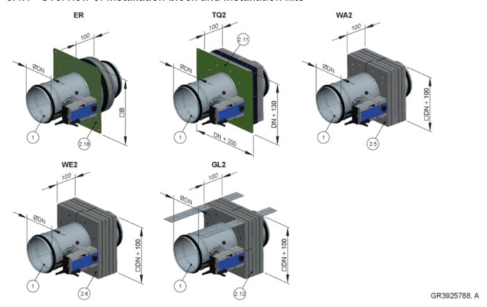
Fig. 28: Overview of installation block and installation kits
