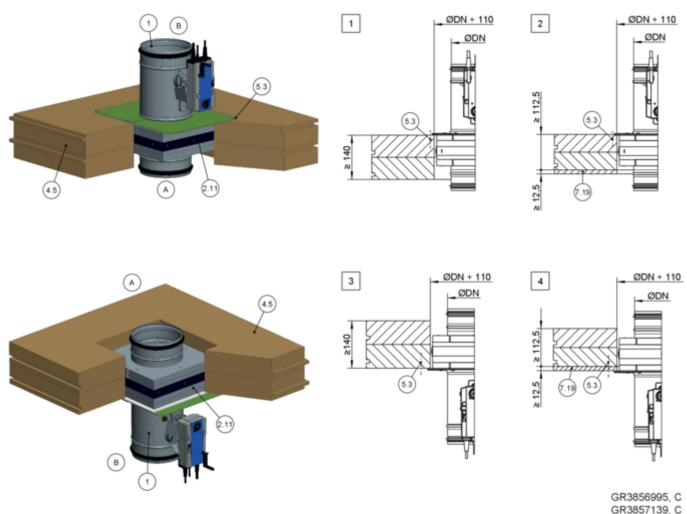
Fig. 172: Dry mortarless installation with installation kit TQ2 into solid wood ceiling, upright and suspended
