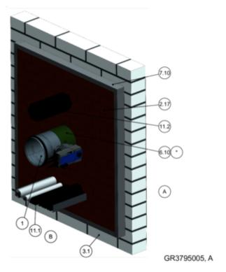
Fig. 26: Fire protection stone bulkhead (mixed execution)
