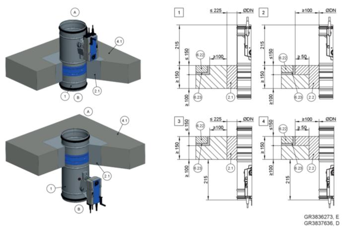
Fig. 146: Mortar-based installation into a solid ceiling slab with screed and footfall sound insulation, suspended or upright
