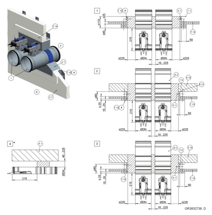
Fig. 135: Mortar-based installation into a shaft wall, flange to flange, illustration shows side by side installation (applies also to installation of dampers on top of each other)
