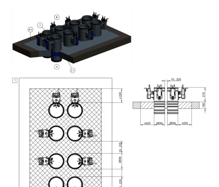
Fig. 150: Mortar-based installation – multiple installation into one installation opening, illustration shows upright installation (applies also to suspended installation)
