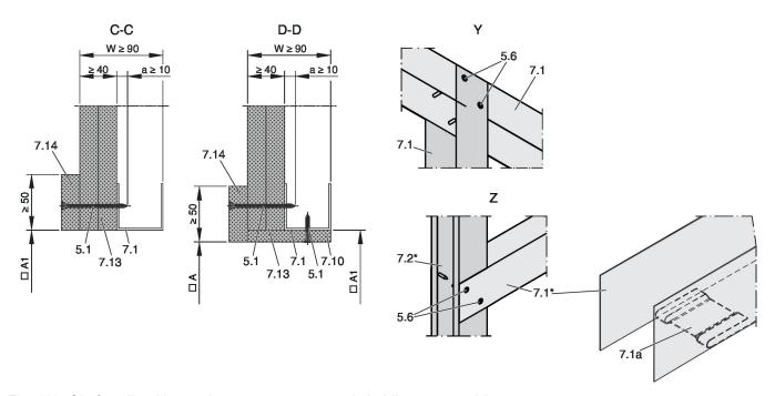
Fig. 132: Shaft walls with metal support structure and cladding on one side
