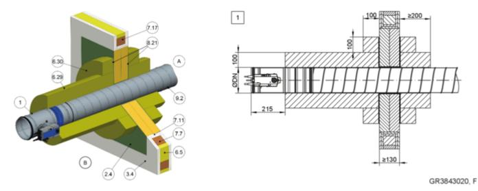
Fig. 114: Dry mortarless installation remote from timber stud walls with mineral wool and fire batt
