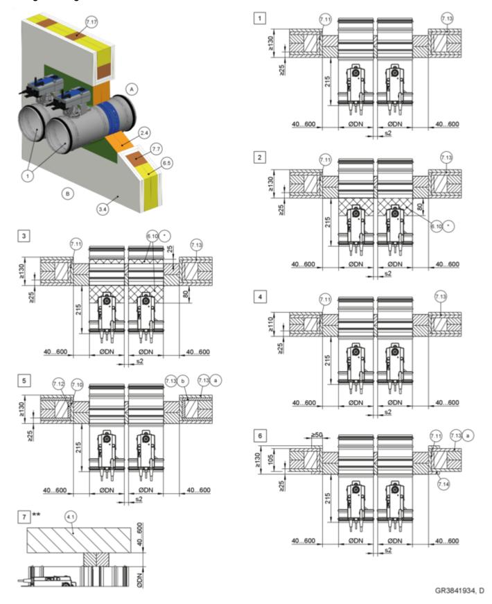
Fig. 117: Dry mortarless installation into a lightweight partition wall with timber support structure, with a fire batt, flange to flange, illustration shows side by side installation (applies also to installation of dampers on top of each other)
