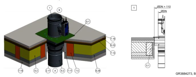
Fig. 163: Dry mortarless installation in lightweight ceiling (ADK modular room system) with installation kit TQ2, drawn standing (also applies to suspended arrangement)
