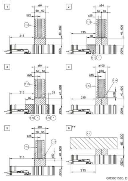
Fig. 96: Dry mortarless installation into a lightweight partition wall, with a fire batt
