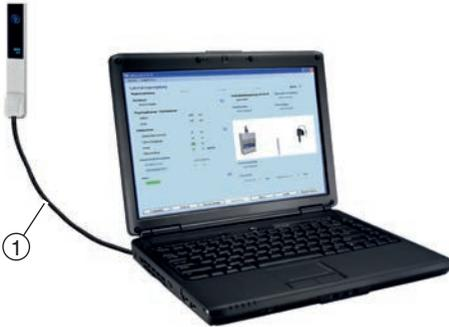
Fig. 7: Connection with the EASYLAB configuration cable
