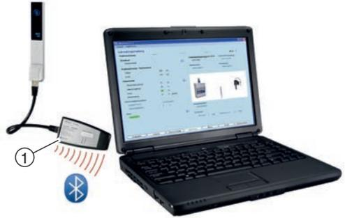
Fig. 8: Connection with the BlueCON Bluetooth adapter
